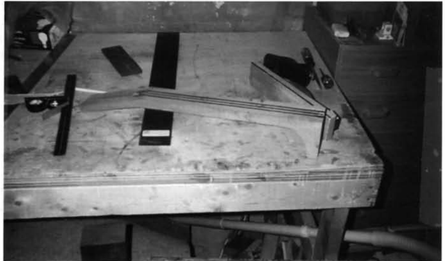
Neck blank with graphite-rod reinforcement.
